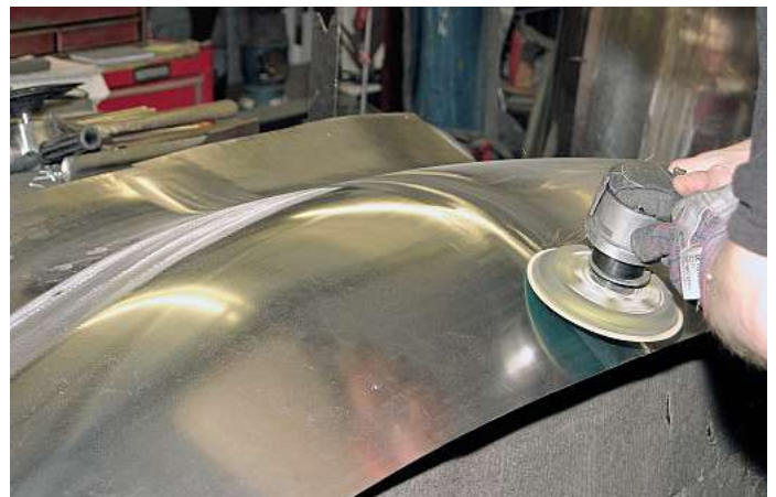
Soothing the curved edges of the double doors. NRM
