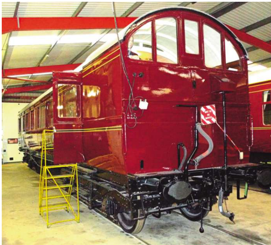
This Lancashire & Yorkshire Railway dynamometer car was used to test locomotives such as the Royal Scot, Princess Royal and Coronation classes. Built in 1912 and original numbered 293, after the Grouping it became LMS No. 45050. Withdrawn in 1967, it is now preserved. ROBIN JONES
