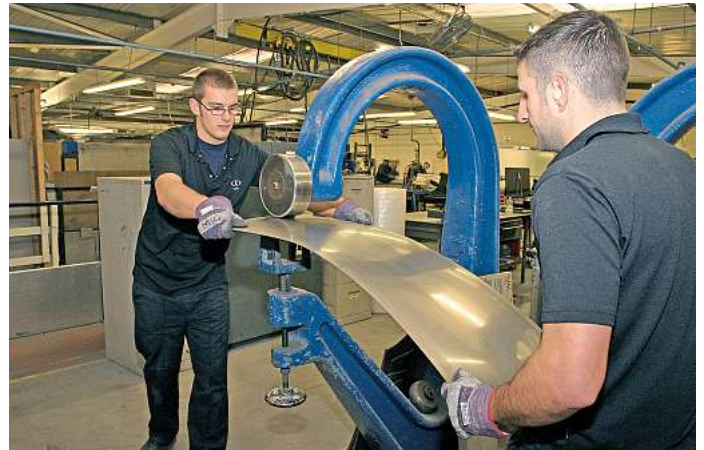
Shaping a curved panel for the front doors. NRM
