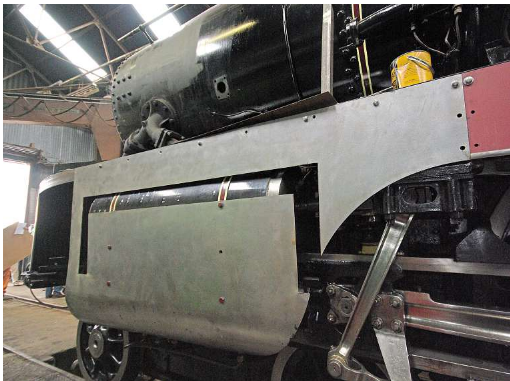
The casing sheet is fitted over the left-hand piston. ROBIN JONES
