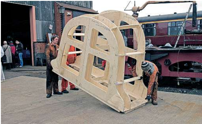
The jig around which the double doors, the most difficult part of the streamlining, were shaped. NRM
