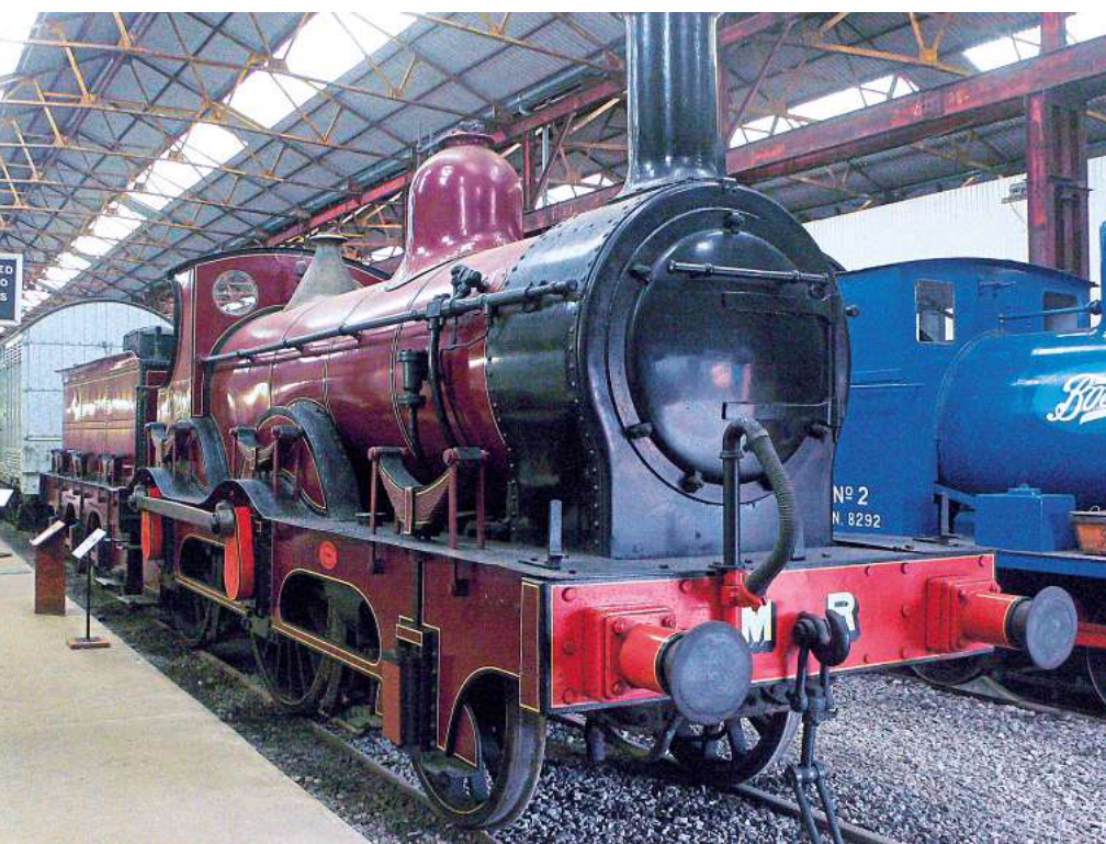
Midland Railway Kirtley 156 class 2-4-0 No. 158A was built in 1866 to a Matthew Kirtley design for express passenger workings to King's Cross, which was then the company's London terminus. The Midland Railway was derided for its small-engines policy, which saw very attractive, polished and superbly presented crimson-lake liveried but small locomotives used on its major routes, often having to double head or rely on banking engines because their individual power was insufficient. No. 158A was rebuilt several times until it was finally withdrawn in 1947 after 81 years service at Nottingham, where it was being used as station pilot. It appeared at the Stephenson Centenary Celebrations in Chesterfield in 1948 and was then preserved at Derby Locomotive Works until moving to the Midland Railway-Butterley in 1975. Part of the National Collection, it is seen on display in the Matthew Kirtley Exhibition Hall at Swanwick Junction. ROBIN JONES
