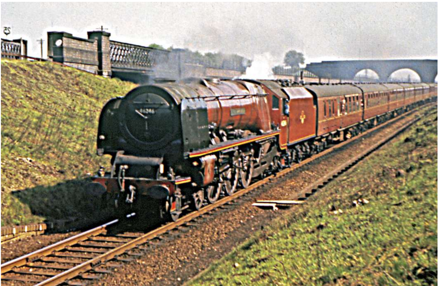
No. 46246 City of Manchester hauls the 'Midday Scot' Glasgow to Euston lunchtime express through Clifton Road Junction in April 1961. Having emerged from Crewe on August 11, 1943, as a streamliner, it underwent six boiler changes and was the last class member to lose its sloping smokebox, in 1960. It was withdrawn on September 12, 1964. COLOUR-RAIL BRM659/D SMITH
