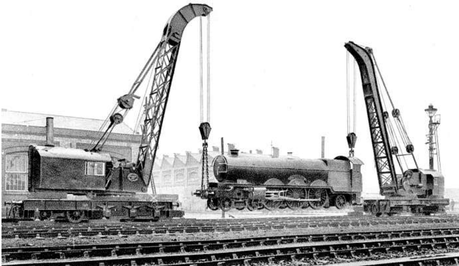
A 36-ton breakdown crane demonstrates its power by lifting Britain's first Pacific, No. 111 The Great Bear . Probably built more for prestige than anything, its designer George Jackson Churchward did not develop the project into a production class. After he retired, he was told that Gresley was planning to build a Pacific for the Great Northern Railway. "What did that young man want to build it for?" he exclaimed. "We could have sold him ours!"
