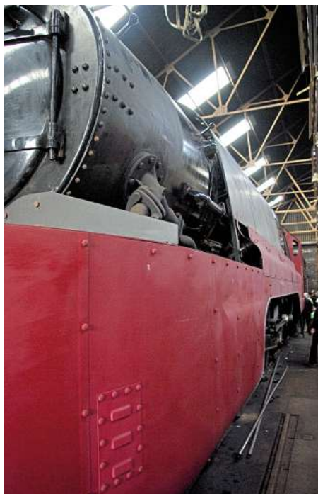
The streamlined casing reaching to the smokebox; all that is now needed are the double front doors. ROBIN JONES
