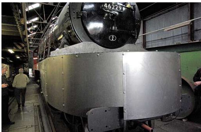
The streamlined casing around the front buffer beam and the platform which will support the two front doors of the housing, as seen on May 26, 2007. ROBIN JONES
