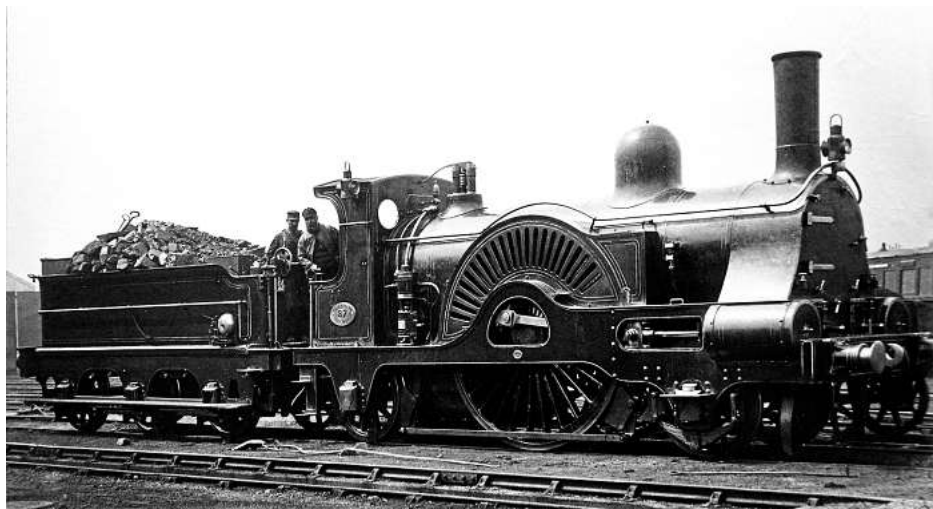
Caledonian Railway 8ft 2in wheeled 2-2-2 No. 87. This class was introduced in 1859 onwards and served as the main express engine until 1885. The last of the class was withdrawn from service in 1901. TONY HISGETT COLLECTION*
