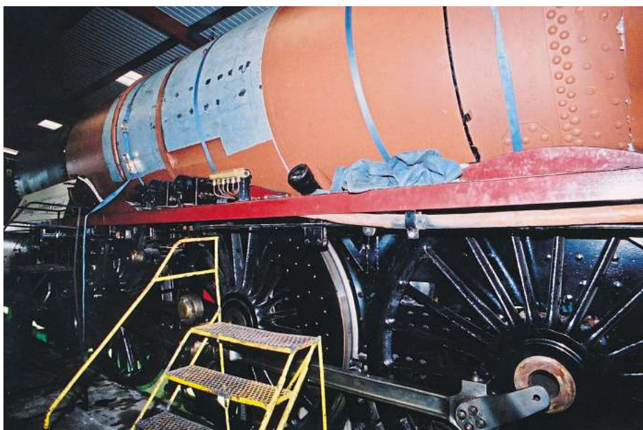
The boiler cladding receives the final touches at the West Shed. ROBIN JONES
