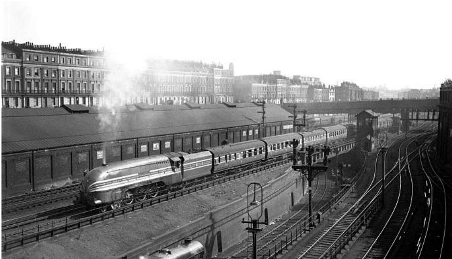
No. 6221 Queen Elizabeth hauling the 'Coronation Scot' up Camden Bank, with Jubilee 4-6-0 No. 5563 Australia backing up towards Camden shed, on September 23, 1938. No. 6221, which came out of Crewe Works on June 14, 1937, four years later became the only blue streamliner to be repainted crimson lake, and was also unique in that it was the only member of the class ever to be equipped with a Princess Royal-type tender without the coal pusher, two years before it was withdrawn on May 18, 1963. NRM
