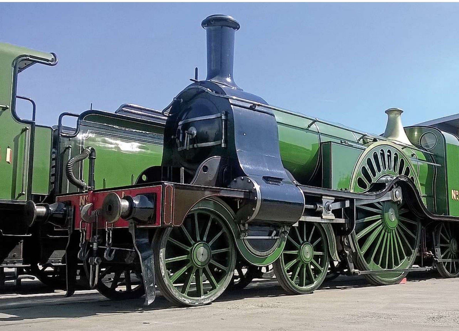
The competition: the Great Northern Railway class Stirling single No. 1 was designed by Patrick Stirling for express passenger work, hauling up to 26 passenger carriages at an average speed of 47mph. Their distinctive feature is a single pair of 8ft driving wheels. The sole-surviving example of a class of 53 built at Doncaster Works, No. 1, is now in the National Collection and is seen outside the Locomotion museum in May 2014, when it was paired again with an original GNR tender which had just been restored. RICHARD PEARSON/LOCOMOTION
