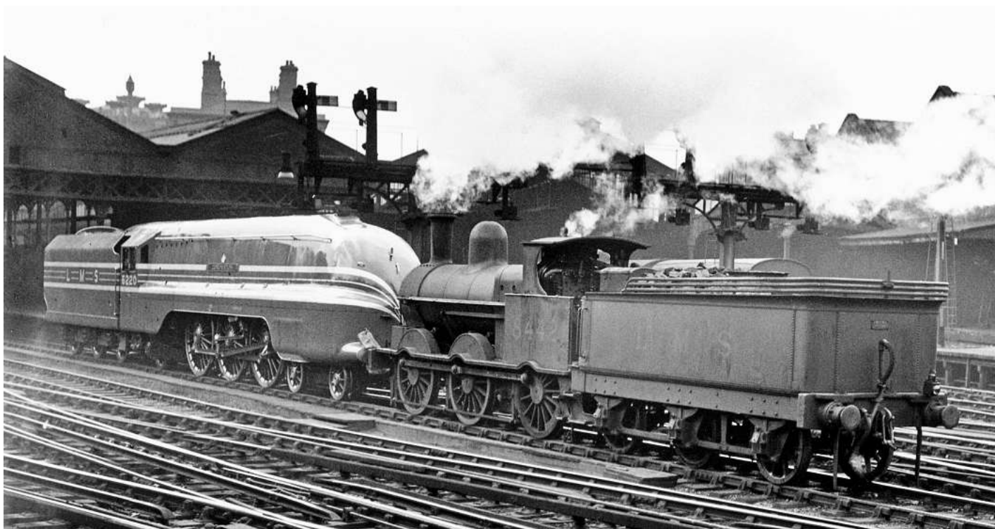
The great adventure begins: the first of Stanier's streamlined Princess Coronation Pacifics No. 6220 Coronation is shunted by LNER 'Cauliflower' 0-6-0 No. 8442 into platform 6 at Euston ahead of the press review trip on June 29, 1937, when the locomotive set a new British speed record of 114mph. The class name celebrated the coronation of King George VI on May 12, 1937. NRM
