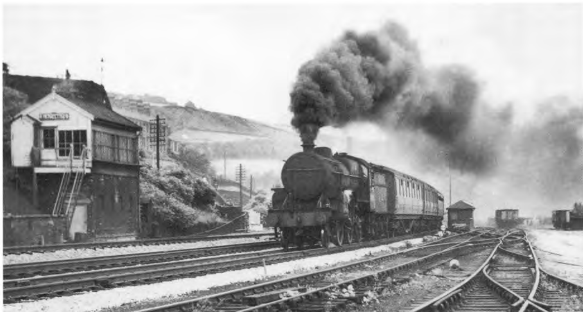
Above: Photographed from Slaithwaite goods yard with the coal yard ahead on the right and the signal box on the left, Farnley Crab 2-6-0 No. 42789 makes a very strong attack on the climb to Standedge with the 9.38am South Shields to Manchester Exchange holiday express at 1.37pm on 9th July, 1960. Despite being loaded to 10 bogies, the Crab was maintaining a pace worthy of much larger locomotives.
