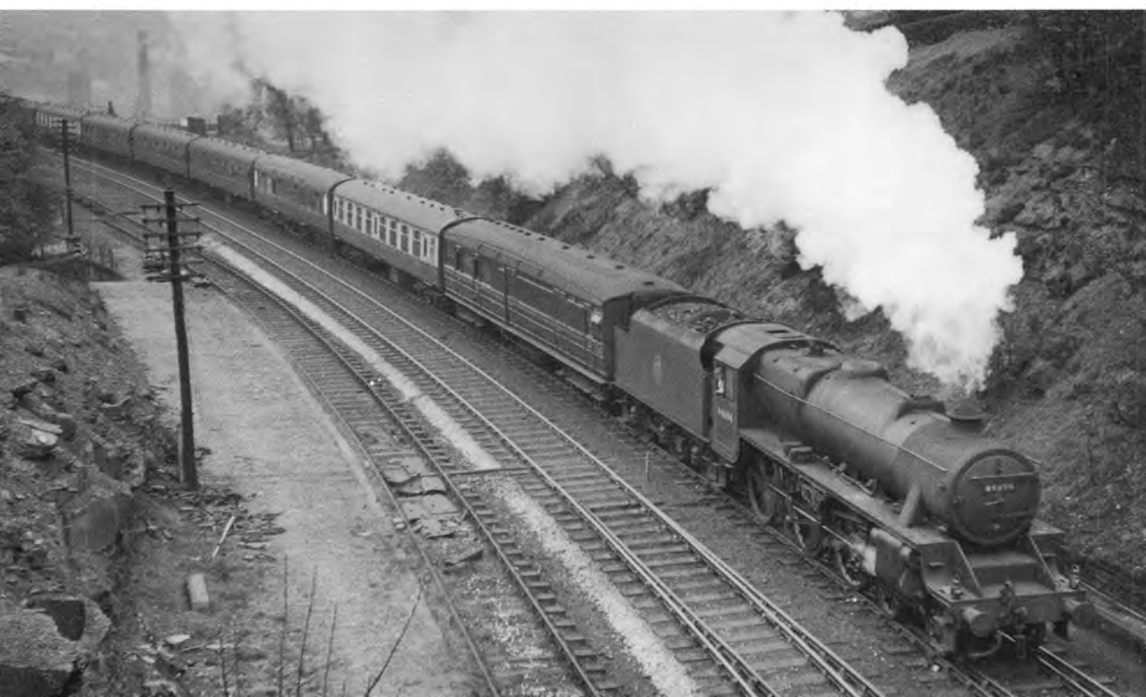
Below: Diverted from the GC Woodhead line by engineering work, the 9.20am Hull-Liverpool Central hauled by Low Moor Black Five No. 44694 approaches Springwood Junction from the Penistone direction on 19th April, 1959. On the left is Springwood coal drops siding, the points to which were controlled by bolt lock from Springwood Junction signal box.
