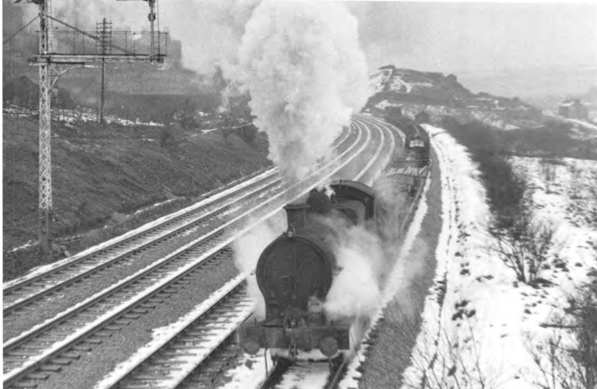
Above: It makes you feel cold just to look at it. A traditional Standedge freight headed by an LNWR Super 'D' 0-8-0 plods up to Longwood & Milnsbridge in February, 1960. Even in BR days, these locos lacked smoke-box number plates.
