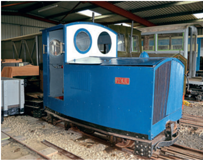
The LCLR is also now home to a similar locomotive to Nocton from the same source, No. 3995 of 1926 Paul . At an early stage during its spell at Humberston, this locomotive was fitted with a 'body' fashioned by a Grimsby boat builder. Note the ex-WDLR 'D' class bogie wagon and bogie ambulance van in the background.
