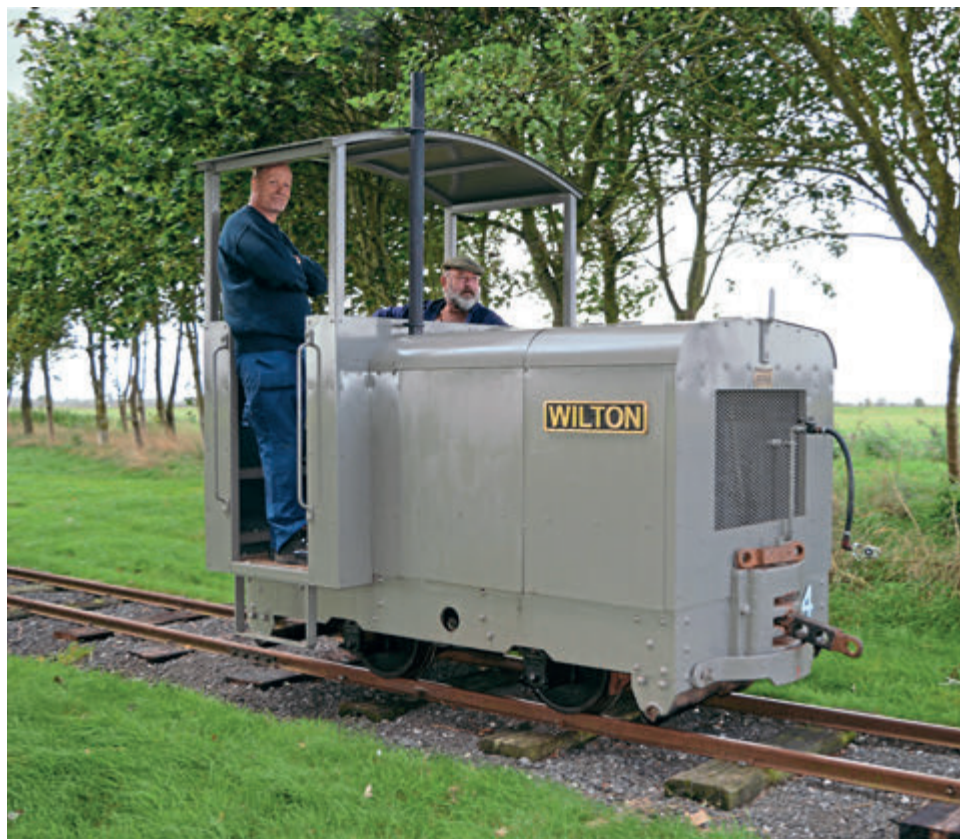
Unlike Gricer , which was constructed to a War Department order, Wilton (Motor Rail No. 7481 of 1940) was originally built for use at Wilton Road brickworks. The pillar cab and rectangular bonnet were fitted in 2015, replacing an earlier body that appears on photographs taken while the engine was at Humberston.
