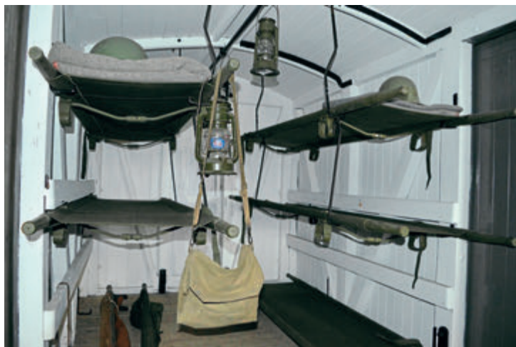
One of the most important features of the resurrected LCLR is the collection of items owned by the LCLR Historic Vehicles Trust, the nucleus of which was a group of ex-WDLR vehicles acquired from the Nocton Estates system. This view shows the restored interior of a bogie ambulance van, complete with stretchers, helmets and other details.
