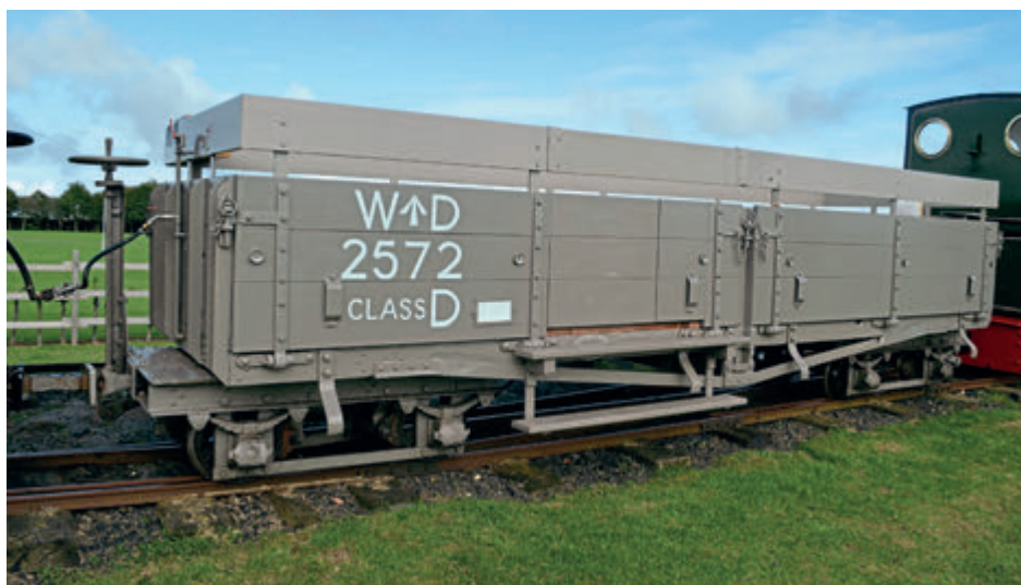
This 1917-vintage Clayton & Shuttleworth 'D' class bogie wagon is owned by the Historic Vehicles Trust and has been given certain modifications (with the aid of National Lottery funding) to enable its use as an accessible open passenger carriage (note the steps and subsidiary door cut into the right-hand portion of the left-hand 'dropside'; also the uppermost safety boards added to the superstructure). Close examination of the solebar and truss-rod areas beneath the centre-left portion of the right-hand 'dropside' reveals ordnance damage received in action during the First World War).
