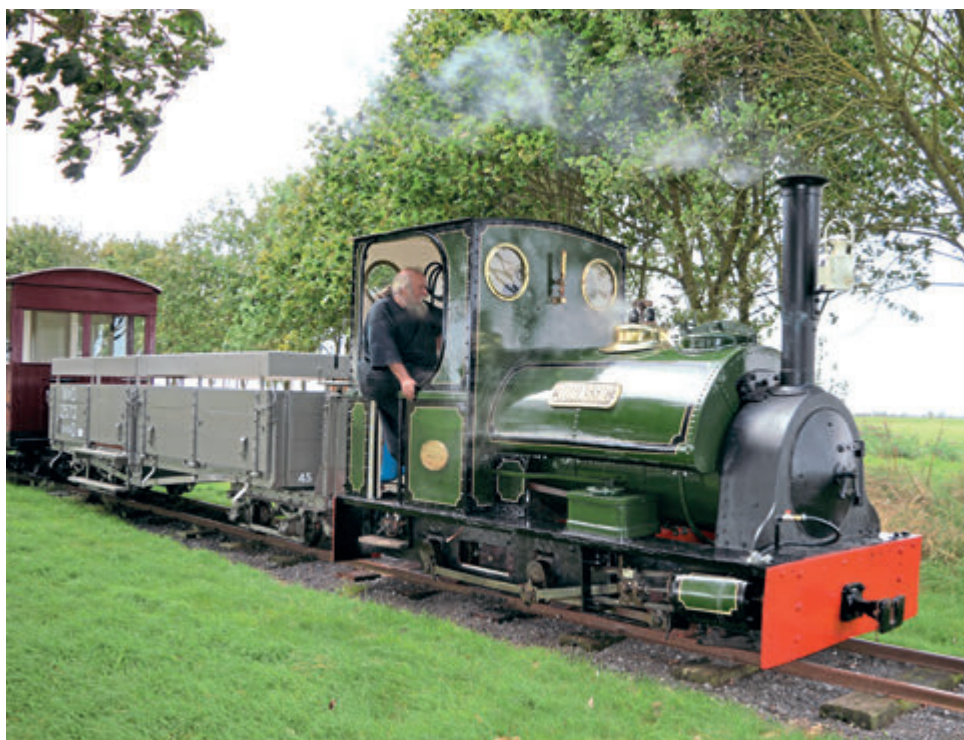
Jurassic and its train are seen from the right-hand side as they approach the Walls Lane area. The air hose, a part of the braking system, can be seen on the right-hand side of the locomotive, immediately behind the bufferbeam, while the steps (for accessibility) on WDLR No. 2572 are visible.
