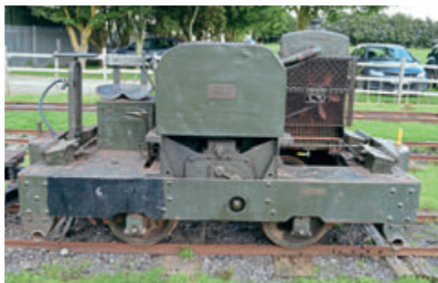
Motor Rail No. 8622 of 1941 Gricer is one of three of the more modern pattern of 'Simplex' 20hp diesel with a straight (as opposed to bow) profile mainframe structure represented on the LCLR.
