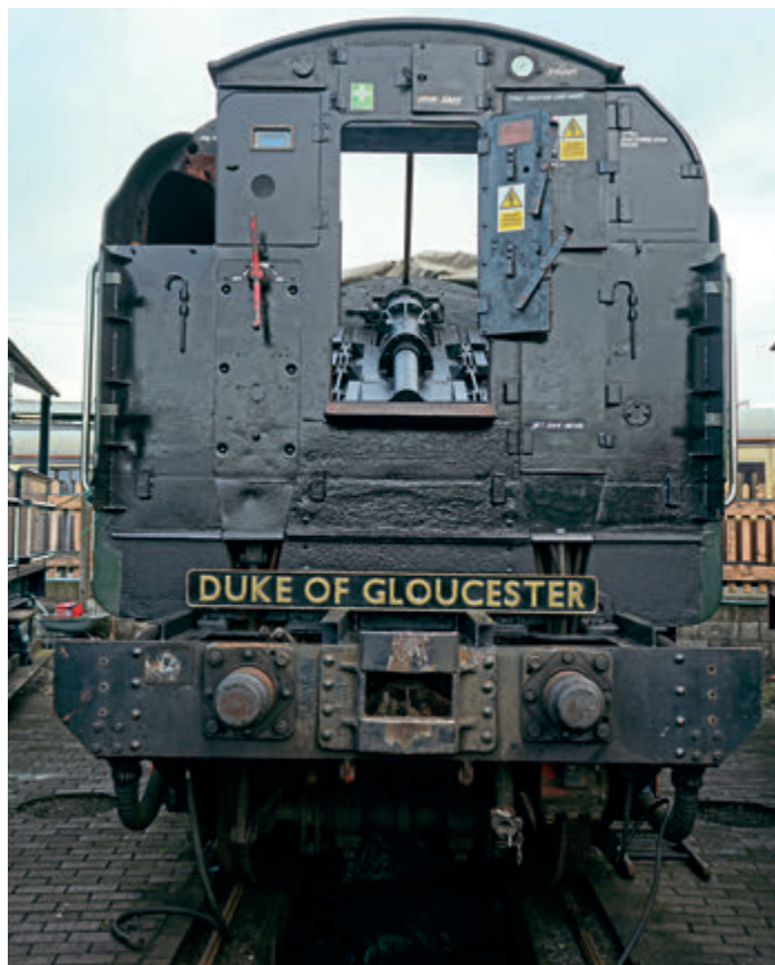
The refurbished tender of No. 71000 Duke of Gloucester with the coal pusher clearly visible. TREVOR TUCKLEY
