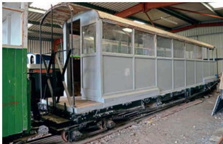
The sole surviving item of rolling stock from the 18in-gauge Sand Hutton Light Railway is the bogie carriage body constructed in 1924 by Robert Hudson & Co. This was acquired by the LCLR in 1967 and mounted on a 2ft-gauge chassis made from two 'D' class underframes. More recently, the carriage suffered from deterioration while in open storage and it has now been moved under cover for remedial work and eventual return to working order.
