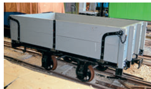
This company-owned 'P' class wagon has been restored in its later condition, as used at Nocton.
