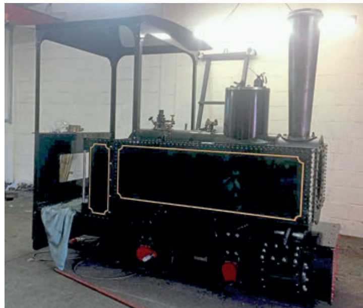
The nearly-complete new-build Decauville 0-4-0T in the NBR Engineering Services workshop. DAVID HUMPHREYS
