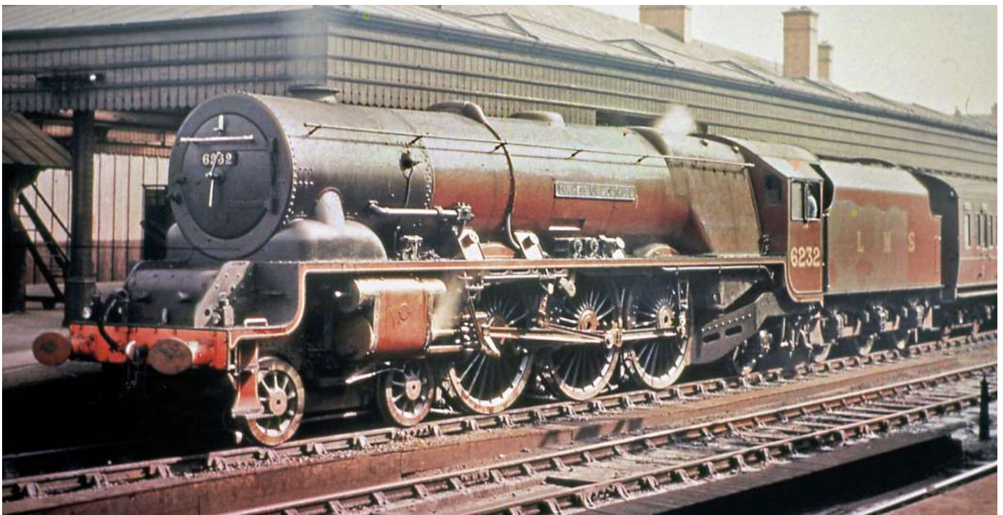
Non-streamlined No. 6232 Duchess of Montrose at Shrewsbury in 1938. No. 6232 was the third of the non-streamliners, outshopped from Crewe on July 1, 1938. It was damaged in a Luftwaffe bombing raid in 1940. When withdrawn on December 29, 1962, it was the only class member still with its original boiler. P WHITEHOUSE/COLOUR-RAIL LM21
