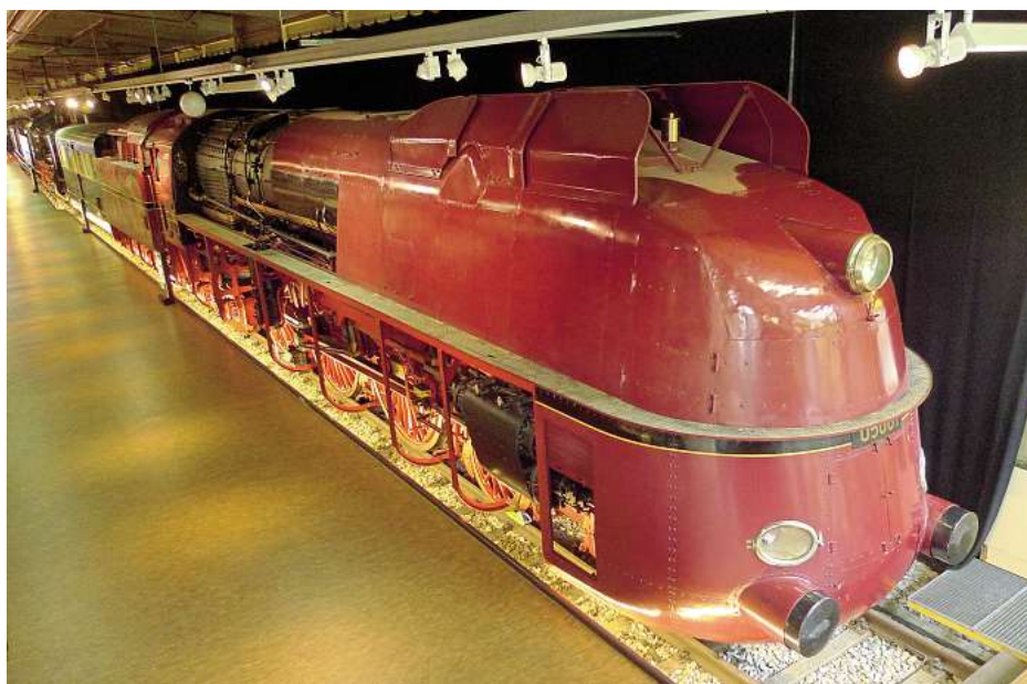
German Class 05 4-6-4 No. 05001, the sole surviving member of a class of three which once included No. 05002, which on May 11, 1936, set a new world steam speed record of 124.5mph. It is displayed inside Nuremberg's Deutsche Bahn Museum. ROBIN JONES
