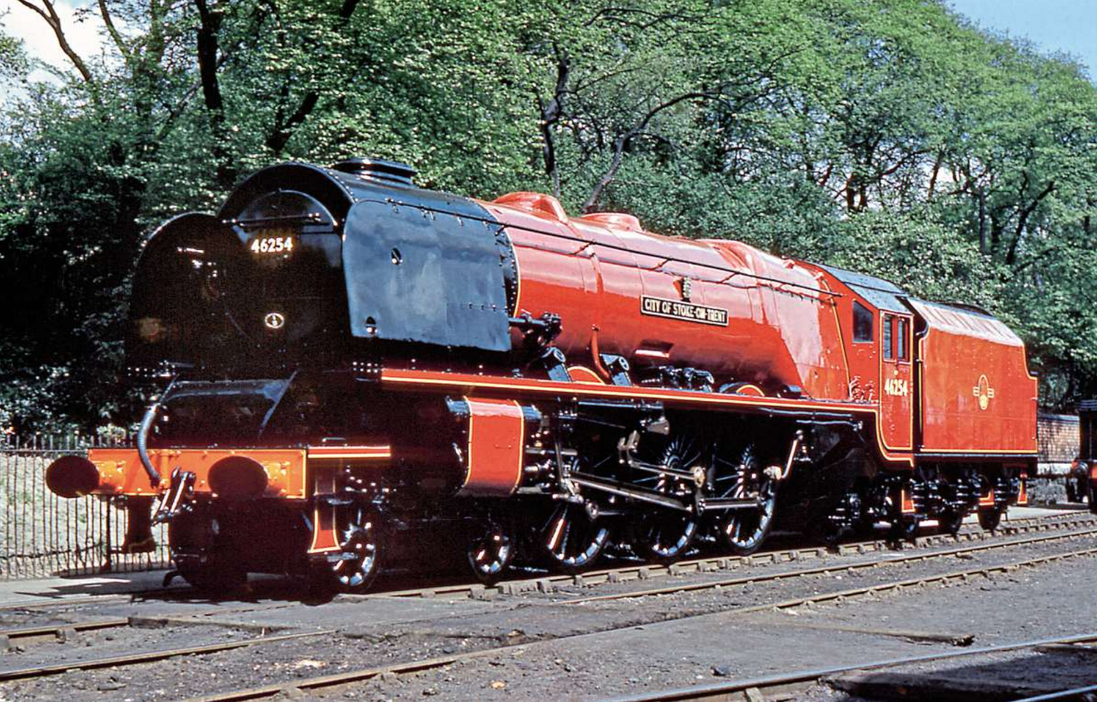
Seen in ex-Crewe Works condition following overhaul, No. 46254 was one of two class members loaned to the Western Region – successor to the GWR where Stanier began his career – in 1956, the other being No. 46257 City of Salford . Outshopped from Crewe on September 17, 1946, it was withdrawn on September 12, 1964. G PARRY COLLECTION/COLOUR-RAIL 312233
