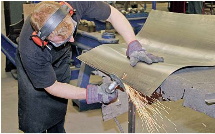
Machining a curved panel for the front casing double doors. NRM
