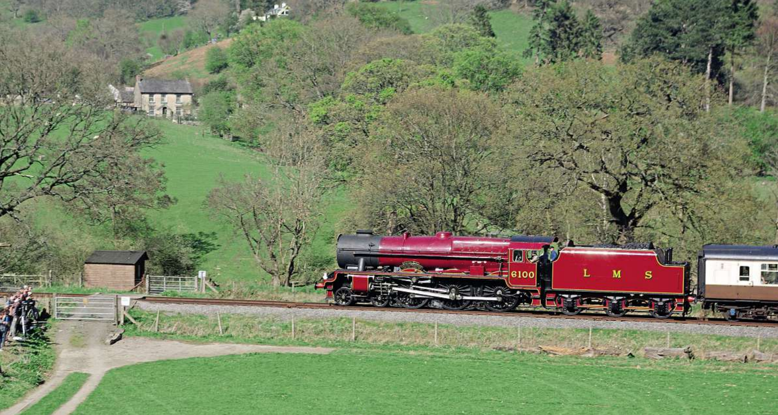
Preserved No. 6100 Royal Scot in action during the Steel, Steam & Stars II gala at the Llangollen Railway in April 2009. The locomotive is running without smoke deflectors, as did the members of the original class until 1931. ROBIN JONES
