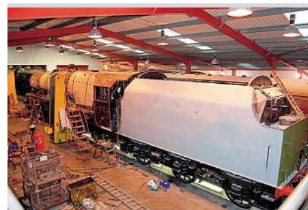
The latest overhaul of No. 6233 rapidly entering its final stages in the West Shed on November 25, 2011. Notice the first coat of green paint on the end of the tender!
