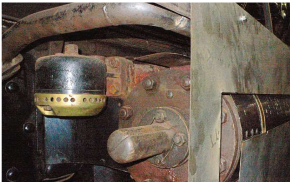
The thinness of the streamlined casing is apparent in this view of the section covering the left-hand piston. ROBIN JONES
