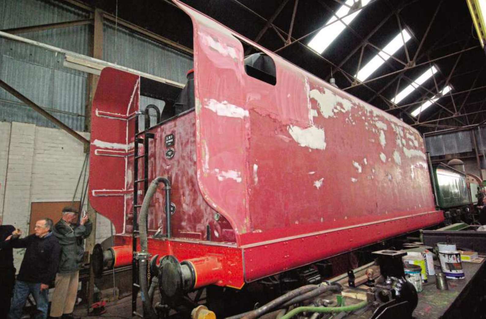
The streamlined tender with fins fitted at the rear. ROBIN JONES
