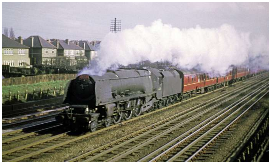
Duchess No. 6253 City of St Albans came out of the works on September 14, 1946. It was the first non-streamliner to have the new 'utility' front footplate together with a cylindrical smokebox, and also the first Duchess with a riveted tender. Seen powering through Kenton in April 1962, it was withdrawn the following January. M SMITH/COLOUR-RAIL BRM2035
