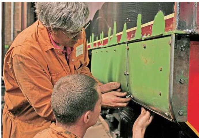
Tyseley's chief mechanical engineer Bob Meanley (left) oversees the trial fitting of the first parts of the streamlined casing. NRM
