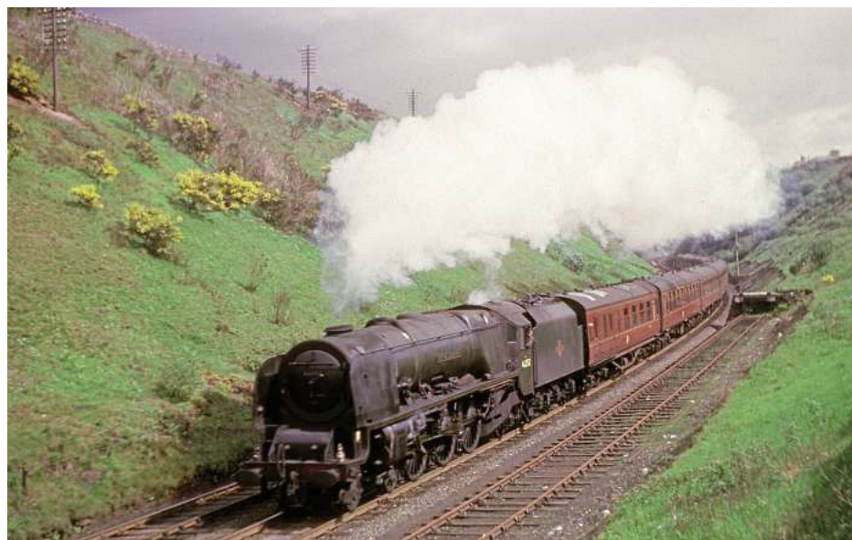
No. 6252 City of Leicester came out of Crewe Works on June 24, 1944, as the last of the four non-streamlined Princess Coronations to be built during World War Two. Seen conquering Shap in June 1962, it was among the first Duchesses to be withdrawn, its career ending on June 1, 1963. M SMITH/COLOUR-RAIL BRM2034
