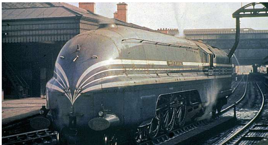
Princess Coronation Pacific No. 6224 Princess Alexandra , the last of the blue streamliners, at Shrewsbury in 1938. Withdrawn in October 19, 1963, it had 11 boiler changes in its career, more than any other member of the class. P WHITEHOUSE/COLOUR-RAIL LM20
